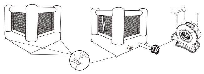
6. Switch blower power on. The product should inflate in approximately 2 minutes. Check for punctures if the product does not inflate properly.
